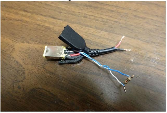
Forcing 4 types of power supply amperages with resistor
